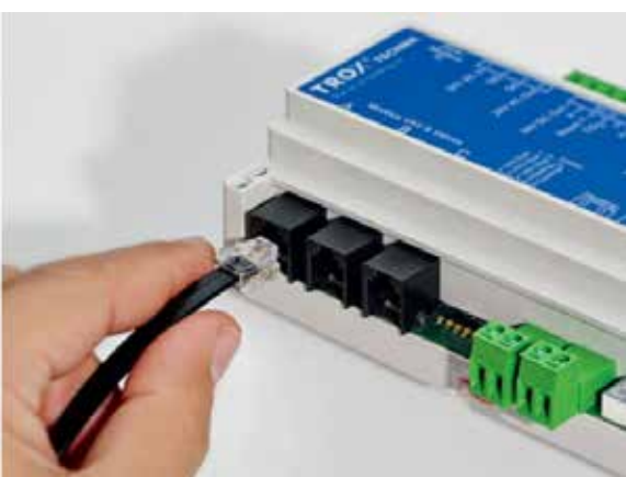
Modbus variant (-J6) with intelligent connection to X-AIRCONTROL
